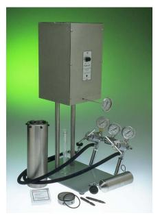
**500 ml HPHT Filter Press** units can be pressurized to 1800 psig on the cell and 750 psig on the back pressure receiver. Maximum operating temperature is 500°F. For operation above 400°F, the filter paper should be backed with a glass fiber filter, or a stainless steel filter.
