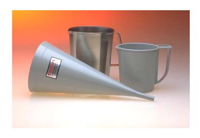
The Marsh Funnel is a simple device for indicating viscosity on a routine basis. When used with a measuring cup the funnel gives an empirical value for the consistency of a fluid. The number obtained depends partly on the effective viscosity at the rate of shear prevailing in the orifice, and partly on the rate of gelation.
