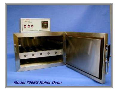
Drilling fluid aging is the process in which a drilling fluid sample, previously subjected to a period of shear, is allowed to more fully develop its rheological and filtration properties. The time period needed to more fully develop properties varies from as little as several hours (usually 16 hours) to as much as several days. Aging is done under conditions which vary from static to dynamic and from ambient to highly elevated temperatures.
