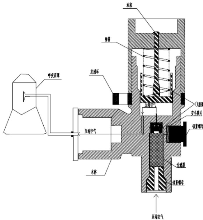
Open the launch belt, and under the action of the spring force, the lifting rod resulting in displacement, corresponding to promote the control of body movement. At this point, cylinder valve is open, compressed air, through the water sealing cap (quantitative hole), enters the filter for decompression, then through the medium-pressure pipe, nose and mouth cover, flows into the mask for the wearer to use.
