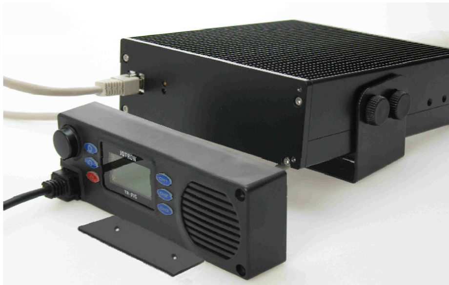
Figure 4.4.3-2, Split desktop mounting
